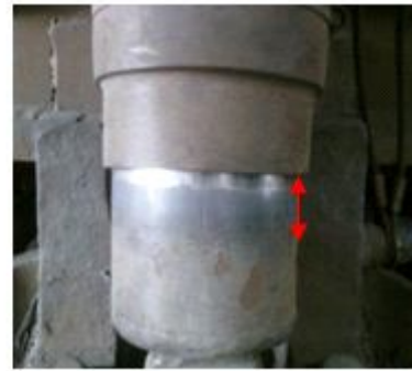
Figure 6. Rubbing marks over inclined damper on end axle
