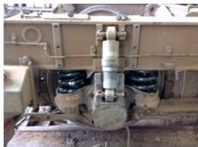
Figure 2. Actual photo of End axle wheel set with Primary spring
