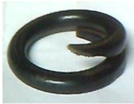
Figure 5. Failed middle axle inner spring
