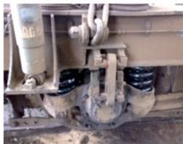
Figure 3. Actual photo of Middle axle wheel set with Composite spring
